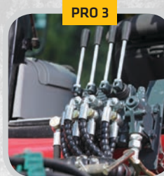
Operated with a control valve. The rotator function is fitted with a float feature so it can free spin when skidding timber.
