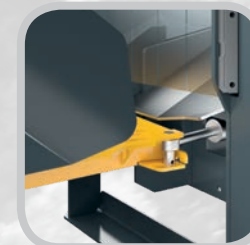
Conveyor belt adjusting position L/R \pm 15^\circ .
