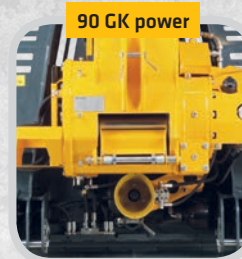
The PTO shaft is installed at the rear side of the winch, enabling a better stability of the tractor and winch and reducing the risk of damaging the cardan shaft.
