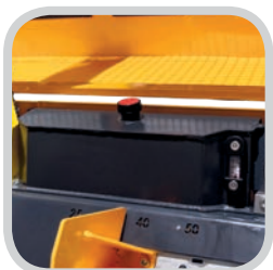
Oil tank for automatic chain lubrication with an oil level indicator.
