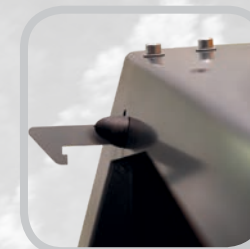
Shutter for retaining the log deck during transport.
