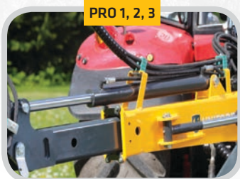
Hydraulic movement left-right (PRO 1, 2, 3). Telescopic arm hydraulic movement (PRO 2, 3).
