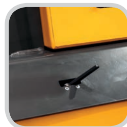
Handle for optional deactivation of log retaining plate.
