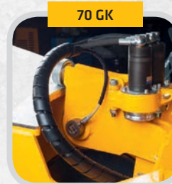
The sensor that measures the pulling force of the winch is directly installed on the pulling rope to enable precise measurement of the force on the pulling rope. The measured pulling rope force is regulated with the clutch. A guide for precise winding of the wire rope on the drum is integrated as standard.
