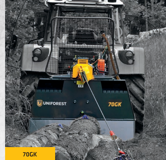
The PTO shaft is installed at the rear side of the winch, enabling a better stability of the tractor and winch and reducing the risk of damaging the cardan shaft.
