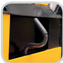
Splitting knife height adjustment handle.
